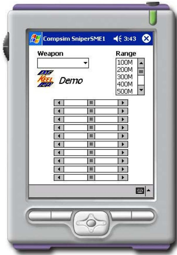
This is a (very preliminary) sample human interface for a Sniper SME demonstration. The weapon / bullet combination could be identified in the combo box in the upper left. The range could be selected from the list box at the upper right. The range would be broken into 10 segments (closest at the top) with windage causing the bullet deflection to show in the horizontal scroll bars. Other inputs from the user will also probably be required.....
